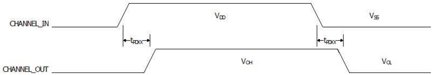
Figure 3: Channel Propagations Delay (/EN = V SS )
